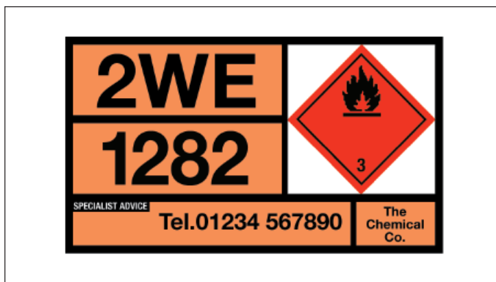
Hazard Warning Panel
