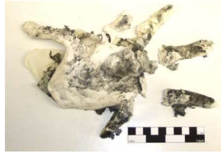
Fig. 4. Unprotected hand surrogate after explosion (plasticine).
