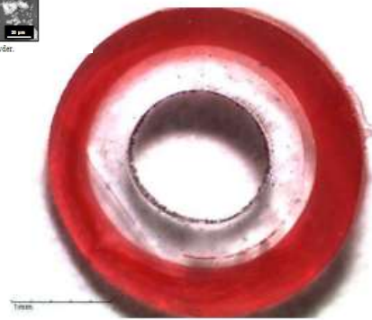
a) shocktube cross section by optical microscope
