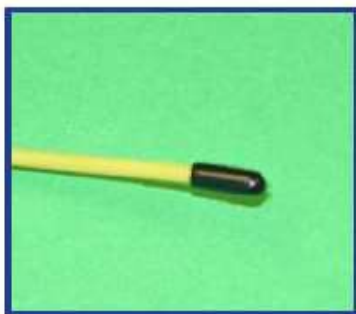
Figure 25 - Cut end of Lead Line covered with vinyl end protector to prevent moisture contamination.
