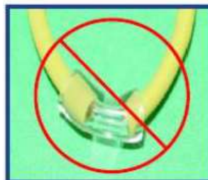
Figure 26 - Incorrect insertion of shock tube into splice. On the left, the splice has been shortened, and on the right the splice has been bent. Both situations could lead to a misfires, which may kill or injure.
