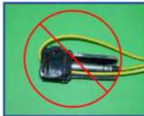
Figure 11 - Shock tube bent around nose of Bunch Block. Cut-off may result.
