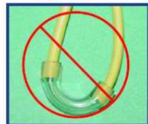
Figure 26 - Incorrect insertion of shock tube into splice. On the left, the splice has been shortened, and on the right the splice has been bent. Both situations could lead to a misfires, which may kill or injure.
