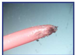
Figure 129 & 130 - Shock tube that has been cut by a pinch-smash break.
