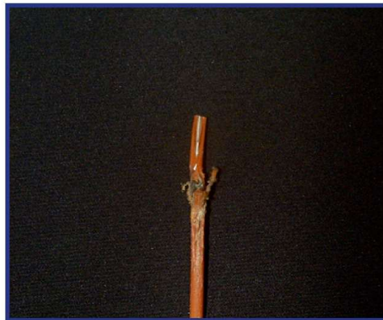
Figure 126 - The cap (removed from this unit) did not function because of the damage shown, which occurred during loading.
