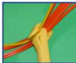
Figure 5 - Six shock tube leads correctly seated in the EZ Connector block.
