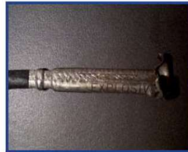
Figure 120 - Detonator after functioning with detonating cord in groove of the connector.
