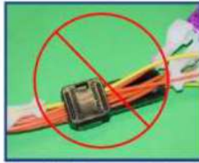
Figure 9 - Shock tube incorrectly inserted into Bunch Block; yellow lead not in direction of initiation.
