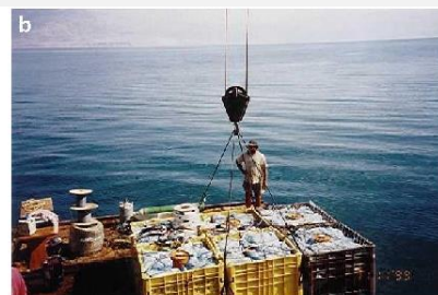
Fig. 2. Sample photographs of the charges of the three explosions: (a) the 500 kg charge unit was used also for the 2060 kg charge; (b) the 5000 kg charge consisted of six units of about 833 kg each.
