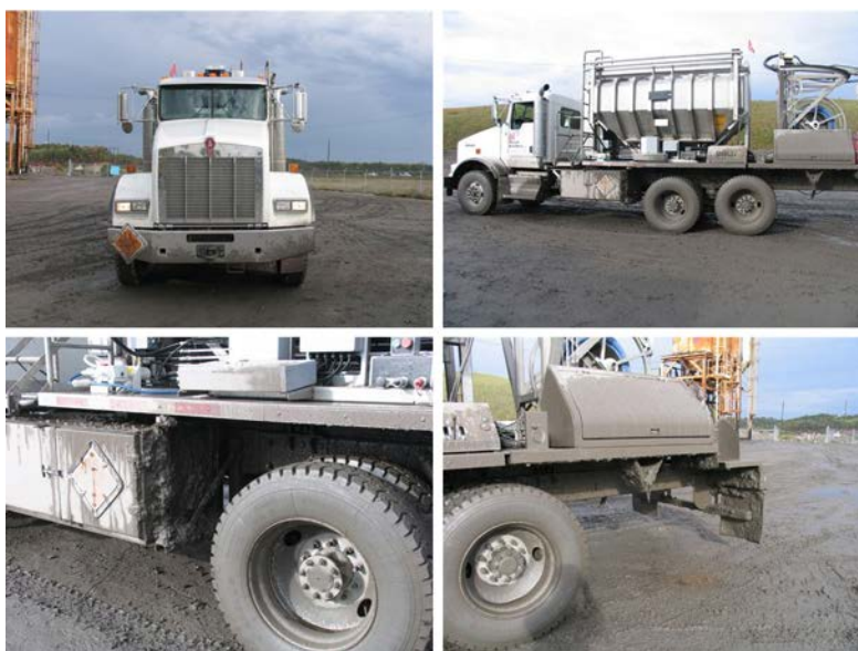
Above: Photograph of bulk truck with 620 pounds of mud as determined by weighing the vehicle clean and dirty
